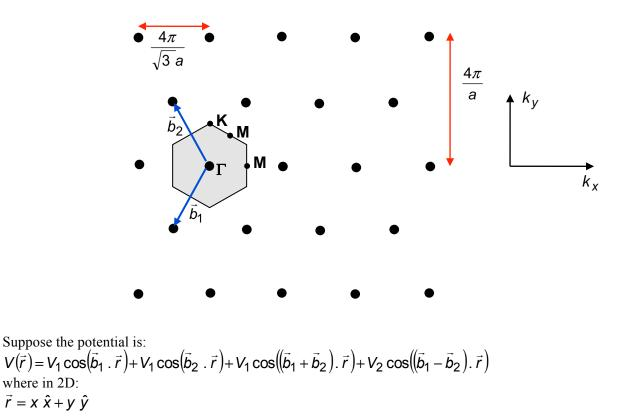
The goal of this problem is to figure out the bandgaps at the K and M points in FBZ using a perturbative approach.
