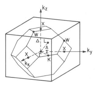
The are 6 equivalent X-points, 8 equivalent L-points, one  $\Gamma$ -point, and 24 equivalent W-points, as shown above. The labeling schemes using alphabets are mostly conventions so you need not worry too much about them.
