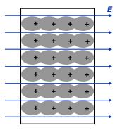
Material gets polarized when placed in an electric field (i.e. develops charge dipoles) because the electron cloud shifts relative to the nuclei
