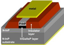
In semiconductor heterostructure laser, the wider bandgap material has smaller refractive index than the narrower bandgap material
