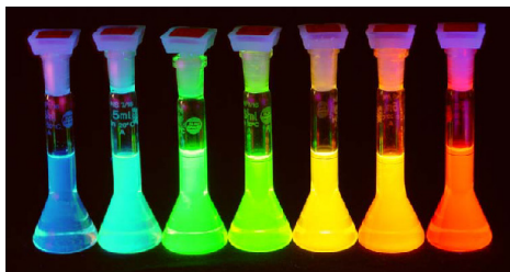
Photoluminescence from CdSe/ZnS (core-shell colloidal) quantum dots of different sizes (~2-6 nm) pumped with the same laser
