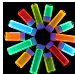
Photoluminescence from CdTe/CdSe (core-shell colloidal) quantum dots of different sizes
