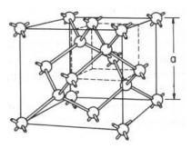
Silicon has a FCC lattice with two basis atoms in one primitive cell
