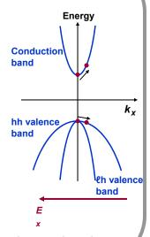
Electrons in the valence band are accelerated in the direction opposite to the force acting upon them due to the applied E-field
