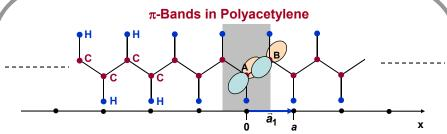
Two carbon atoms per primitive cell implies we have a 1D crystal with a two-atom basis with basis vectors:
