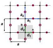
$$E_{SA} c_{SA}(\bar{k}) - 4V_{SS\sigma} \cos(\bar{k}.\bar{d}_1)\cos(\bar{k}.\bar{d}_2)c_{SB}(\bar{k}) = E(\bar{k})c_{SA}(\bar{k})$$
