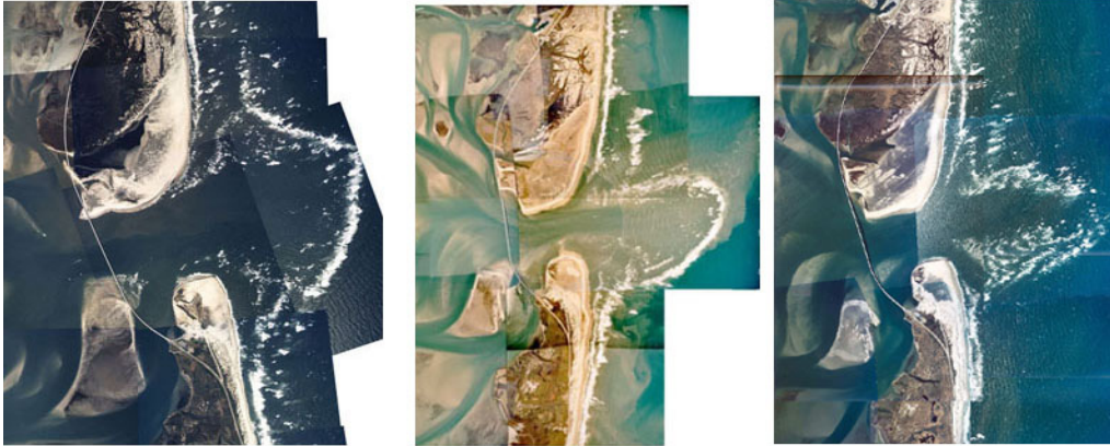
Figure 3. Aerial photography at Oregon Inlet, NC in 1999, 2001, and 2003. Note the changing shape of the ebb shoal as the inlet narrows and ebb currents become more dominant.
