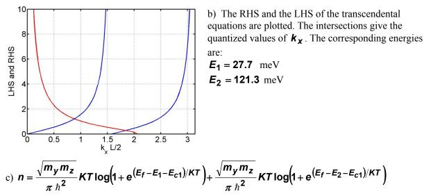
d) Assume T=300K (room temperature). Plot the RHS as a function of the Fermi level and see which value of the Fermi level gives you the electron density on the LHS. This method yields  $E_f - E_{c1} = 53.4$  meV.
