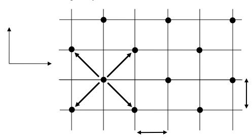
Each atom has a mass **M**. The crystal has a bond-stretching force constant of  $\alpha$ .
