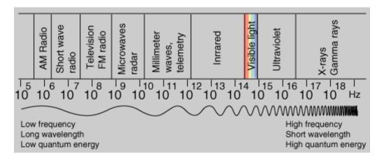
b) In a doped semiconductor, the electron density is  $10^{17}$  1/cm<sup>3</sup>. Assume the dielectric constant of the semiconductor to be  $\mathcal{E}_0$ . Find the plasma frequency  $\omega_p$  of this semiconductor, convert it into Hertz, and then using the figure below find in which part of the electromagnetic radiation spectrum (i.e. am radio, infrared, etc) does it fall. **Be careful that you don't mix up the units.**
