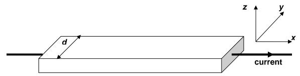
The metal has an electron density equal to n, and an electron scattering time  $\tau$ . A uniform magnetic field in the z-direction, given by  $\bar{B} = B_0 \hat{z}$ , is applied to the sample. In addition a uniform electric field in the x-direction, given by  $E_x$ , is also applied by connecting the sample to an external voltage/current source via leads, as shown. In the presence of the fields, the total force on the electrons is given by the Lorentz expression:
