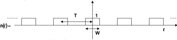
Find the Fourier transform  $h(\omega)$  of h(t) and show that it consists of a train of delta functions with unequal weights. **Hint:** write h(t) as a convolution of the functions in parts (a) and (b). **Lesson:** The Fourier transform of a periodic function consists of only certain discrete frequencies.
