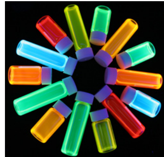
Photoluminescence from CdTe/CdSe (core-shell colloidal) quantum dots of different sizes
