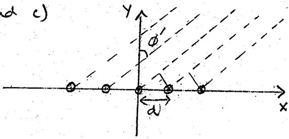
In the  $\phi'$ -direction, if the path difference between the waves emitted from adjacent dipoles is a multiple of the wavelength  $\lambda$  then the waves from adjacent dipoles will add in phase.
